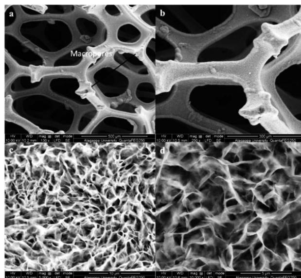
Fig. 2 FE-SEM images of NiCo-MOF/NF at various scales: (a) 500  $\mu\text{m}$ , (b) 300  $\mu\text{m}$ , (c) 10  $\mu\text{m}$ , and (d) 5  $\mu\text{m}$ .
