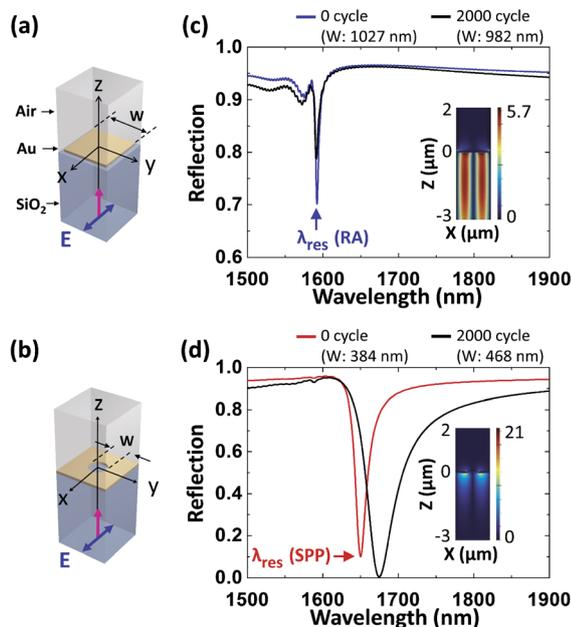
Fig. 5 Schematic of 3D unit cell simulation models for (a) square Au nanopatch array and (b) circular Au nanohole array ( $P = 1100$  nm). Simulated reflection spectra of (c) the square Au nanopatch array and (d) circular Au nanohole array before thermal loading and after 2000 cycles of thermal loading. The insets show the electric field distributions ( $|E_z|$  at  $y = 0$ ) at the  $\lambda_{\text{res}}$  before thermal loading.
