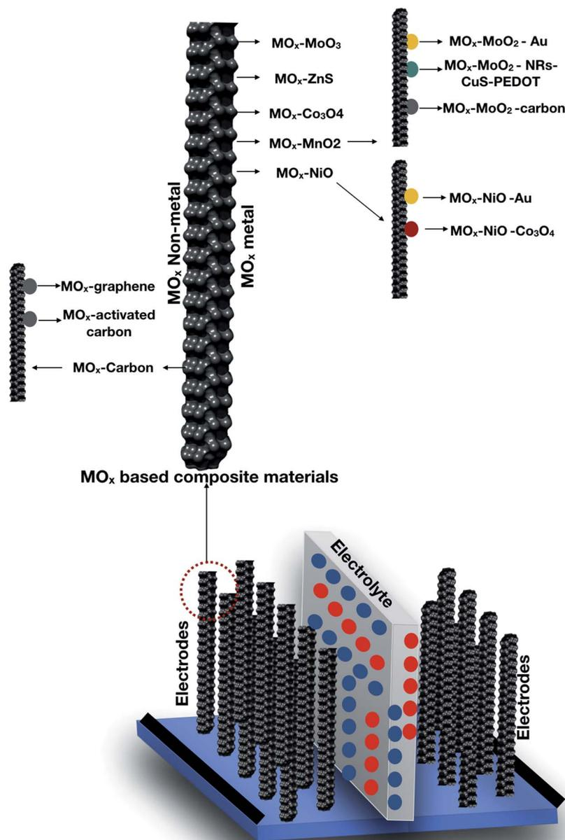
Fig. 21 Metal oxide (MO<sub>x</sub>) based composite materials for advanced supercapacitors, including composites doped with metal and nonmetallic materials.
