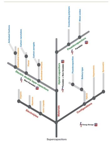
Fig. 2 An overview of the taxonomical classification of supercapacitors. The lightning bolt symbol represents energy and the cylindrical stack represents the storage.
