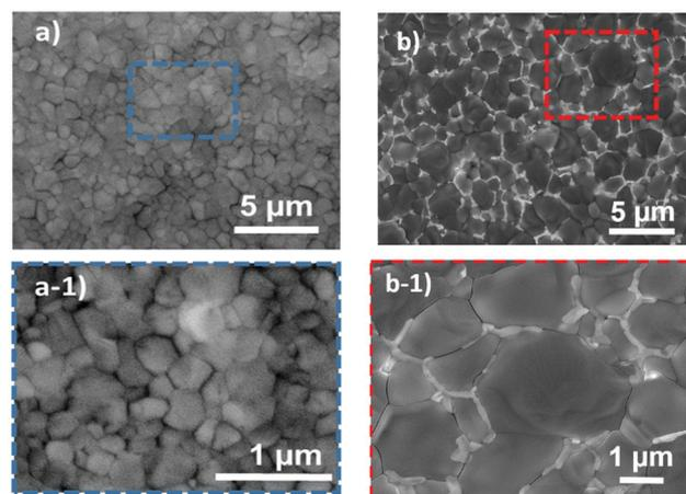
Fig. 1 SEM images of the perovskite films without the additive SOL-0 (a and a-1) and with 5.8 wt% of the additive (SOL-5.8) (b and b-1).
