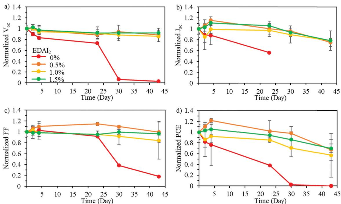
Fig. 6 Normalized (a)  $V_{oc}$ , (b)  $J_{sc}$ , (c) FF, and (d) PCE of the devices containing the active layers of (CsGA)<sub>15</sub> + 0–1.5% EDAl<sub>2</sub> over time in a nitrogen-filled glove box. The (CsGA)<sub>15</sub> + 0% EDAl<sub>2</sub> devices showed a short-circuited behavior after 30 days.
