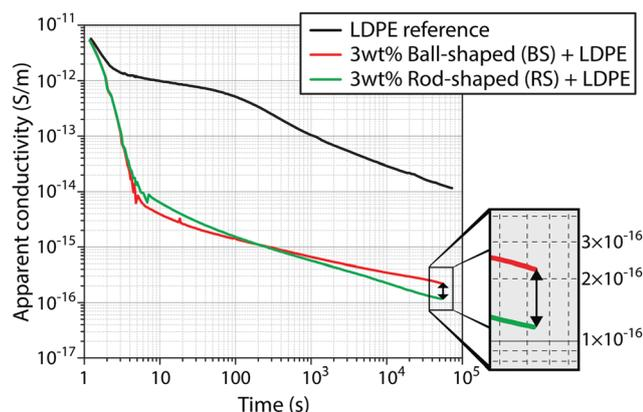
Fig. 2 Apparent conductivity of composites containing 3 wt% ball- or rod-shaped particles and of pristine LDPE at 30 kV mm<sup>-1</sup> at 60 °C. Several measurements up to 2 days were made independently on separately prepared samples, see Fig. S2 (ESI<sup>†</sup>).
