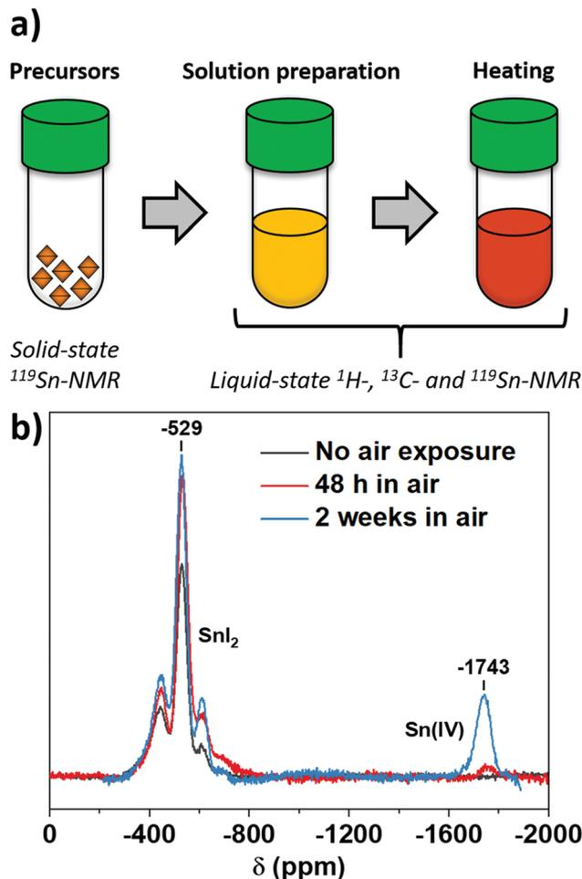
Fig. 1 (a) Steps of tin-based perovskite material preparation studied in this work as possible sources of Sn(II) oxidation; (b) solid-state  $^{119}\text{Sn}$ -NMR spectra of  $\text{SnI}_2$  precursor with and without air exposure.
