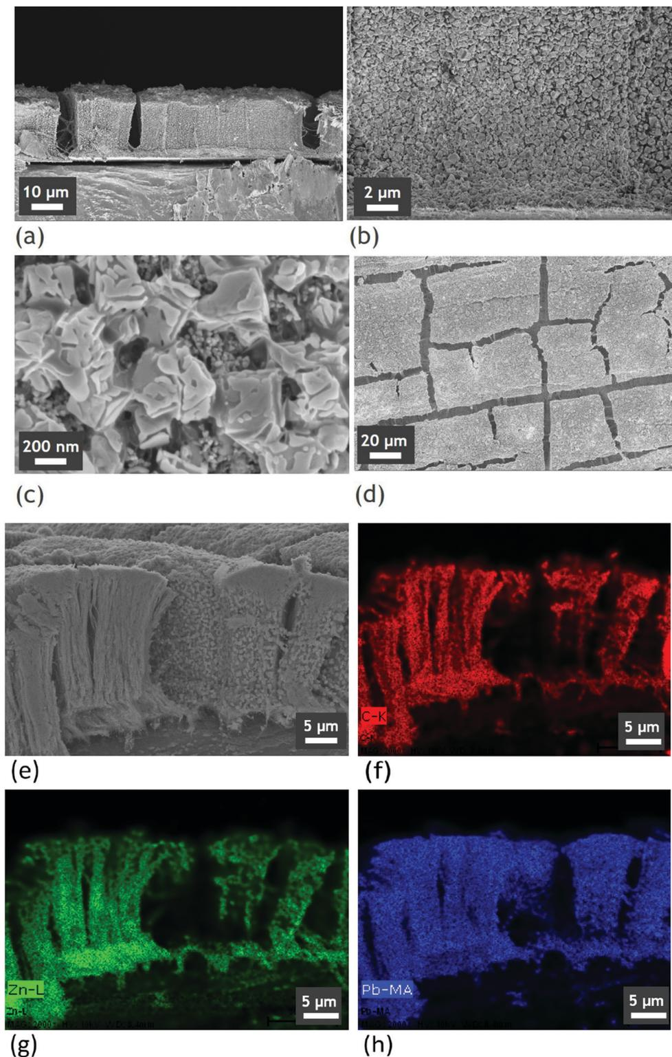
**Fig. 4** (a–c) SEM cross-section views at different magnifications of Al/VACNT/ZnO/perovskites and (d) top view of the deposit. (e) SEM cross-section of Al/VACNTs/ZnO/perovskite and associated EDX analysis. (f) Carbon repartition, (g) Zn repartition and (h) Pb repartition. These pictures show the efficient colocalization of CNTs, ZnO and perovskite.
