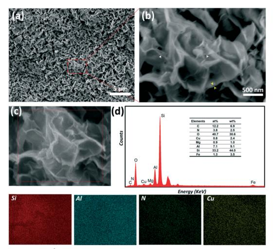
Fig. 3 (a) and (b) SEM images of Cu<sup>2+</sup>@POSS\_SWy-2. (c) SEM image with the area selected for energy dispersive X-ray spectroscopy (EDS) spectra and EDS elemental mapping measurement marked in red. (d) SEM-EDS spectra of Cu<sup>2+</sup>@POSS\_SWy-2. Inset: The elemental composition results. The bottom panels show the EDS elemental mapping results for Si, Al, N and Cu in Cu<sup>2+</sup>@POSS\_SWy-2 based on the red square area in (c).
