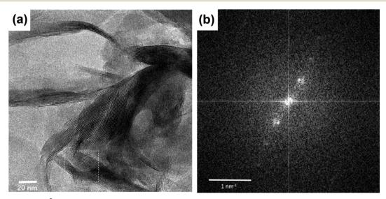
Fig. 2 (a) TEM image of Cu<sup>2+</sup>@POSS\_SWy-2. (b) Fast Fourier transform (FFT) of the square marked in white. An interlayer distance of 17.9 Å is deduced from this graph.
