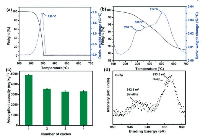
Fig. 6 Thermogravimetric analysis (TGA) and differential thermal analysis (DTA) data for (a) chloridazon and (b)  $Cu^{2+}$ @POSS\_SWy-2 + chloridazon, and (c) adsorption capacity for chloridazon of  $Cu^{2+}$ @POSS\_SWy-2 after an increasing number of thermal regeneration cycles. (d) X-ray photoelectron spectrum of the  $Cu^{2+}$ @POSS\_SWy-2.
