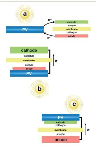
Fig. 1 Plausible schemes for the conversion of sunlight,  $CO_2$  and  $H_2O$  to fuels based on a PV plus unbiased electrolyser architecture: a) simple wired PV plus an electrolyser; b) and c) integration of the PV module as a support for a cathode or an anode, to drive both reactions through the wired counter electrode.
