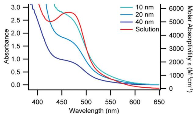
**Fig. 1** UV-Vis absorbance of **3** in  $\text{CH}_2\text{Cl}_2$  (red, right axis) and immobilized in AAO pores of various pore size (blue traces, left axis), constant path length.
