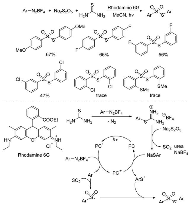
**Scheme 2** Photoinduced three-component reaction of aryldiazonium tetrafluoroborates, sodium metabisulfite and thiourea.
