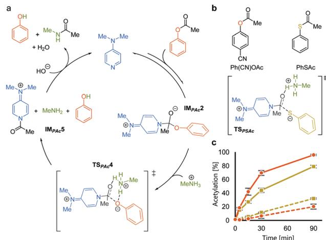
**Fig. 2** Mechanistic analyses of DMAP-catalyzed acetylation with PAc. (a) A plausible catalytic cycle based on DFT calculations. (b) Comparison between phenyl acetate and phenyl thioacetate. (c) Reaction profiles of the acetylation of **7** (solid lines) and **8** (dotted lines) using Ph(CN)OAc (●) and PhSAc (■) at 30 °C.
