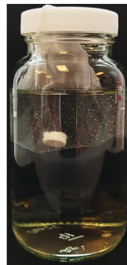
Fig. 4 PNA65-50 cylindrical aggregate nanogel implant held inside 150 µm pore size mesh bag suspended in release media.
