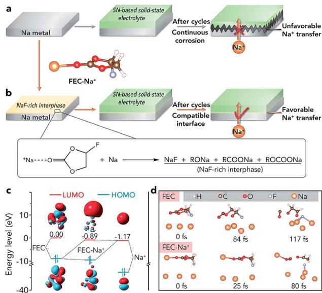
Fig. 1 Schematic diagram of the compatibility between different Na metals and SN-based SSEs: (a) pristine Na metal, (b) 1 M NaClO<sub>4</sub>/FEC modified Na metal; the inset is the chemical reaction between FEC-Na<sup>+</sup> and Na metal. (c) The energy levels/plots of the LUMO and highest occupied molecular orbital (HOMO) of FEC, Na<sup>+</sup>, and FEC-Na<sup>+</sup>. (d) *Ab initio* molecular dynamics models of the reactions between Na metal and FEC (top) or FEC-Na<sup>+</sup> (bottom).
