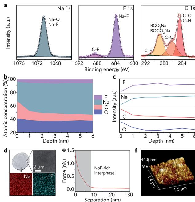
Fig. 2 Characterization of the *in situ* formed NaF-rich interphase on the surface of Na metal. (a) High-resolution XPS spectra of Na 1s, F 1s, and C 1s, (b) atomic percentages and (c) relative elemental intensities at different depths, (d) optical photograph, SEM image, and elemental maps (Na and F), (e) retracted force–distance curve, and (f) AFM topography image with a 3D view.
