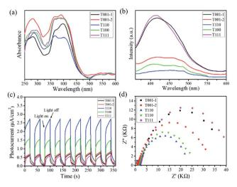
Fig. 3 (a) UV-visible diffuse reflectance spectra, (b) PL emission spectra, (c) photocurrent responses, and (d) EIS Nyquist plots for NH<sub>2</sub>-MIL-125(Ti) with different morphologies.
