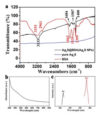
**Fig. 2** Optical adsorption and photodynamic properties of  $Ag_2S$  NPs. (a) FT-IR spectra of  $Ag_2S$ @BSA ( $Ag_2S$  NPs), BSA and pure  $Ag_2S$ . (b) UV-vis spectrum of  $Ag_2S$  NPs (3.5  $\mu g$  ml<sup>-1</sup>) in aqueous solutions. (c) Fluorescence spectrum of  $Ag_2S$  NPs (3.5  $\mu g$  ml<sup>-1</sup>) in aqueous solution.
