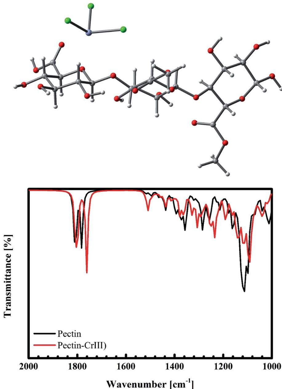
Fig. 19 *Ab initio* simulation of the interaction between Cr(III) and pomelo fruit peel.
