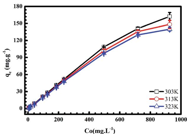
Fig. 6 Effects of initial concentration on the adsorption of MB onto pomelo fruit peels.
