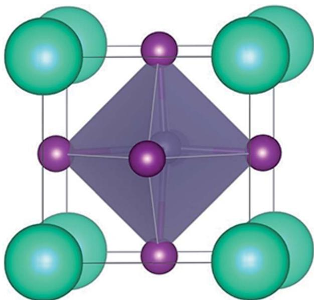
Fig. 1 The crystal structure of CsGeI<sub>3</sub>.
