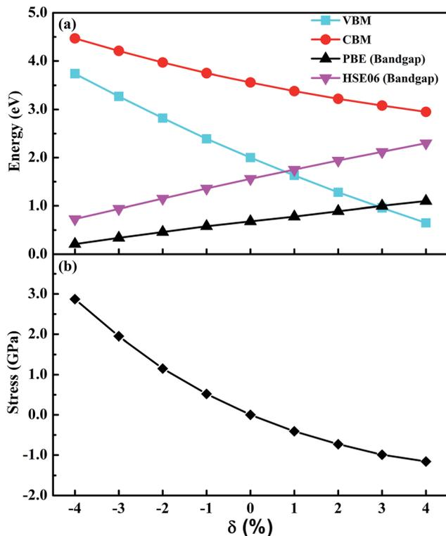
Fig. 4 (a) VBM, CBM, bandgap and (b) stress of CsGeI<sub>3</sub> as a function of strain.
