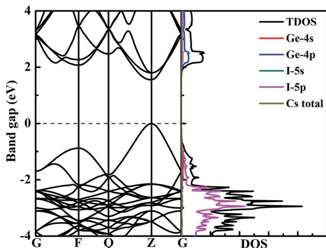
Fig. 3 The band structure and density of states of CsGeI<sub>3</sub> calculated at the HSE06 level.
