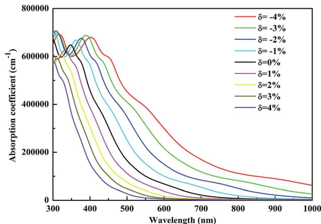
Fig. 7 Calculated optical absorption coefficients of CsGeI<sub>3</sub> under different strain conditions.
