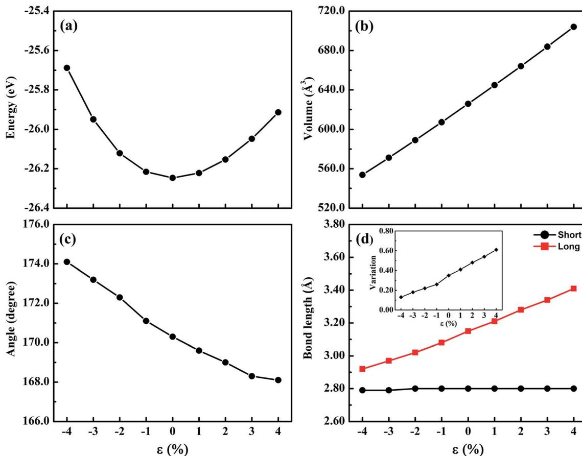
Fig. 2 The structural parameters of CsGeI<sub>3</sub> under different strain conditions. (a) The curve of energy. (b) The curve of volume. (c) The curve of the Ge–I–Ge angle. (d) The curve of the Ge–I bond length. The variation of the short and long Ge–I bond lengths is shown in the inset of (d).
