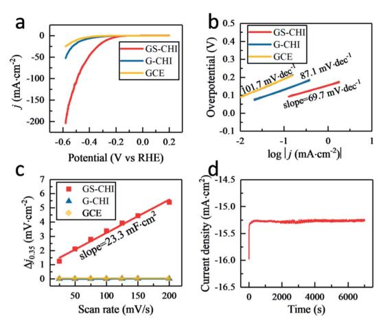
Fig. 4 (a) LSV curves of GS-CHI, G-CHI and blank GCE; (b) Tafel plots of GS-CHI, G-CHI and blank GCE; (c) capacitive current as a function of scan rate for GS-CHI fitted to a linear regression; (d) durability of GS-CHI at -300 mV potential for 7000 s.
