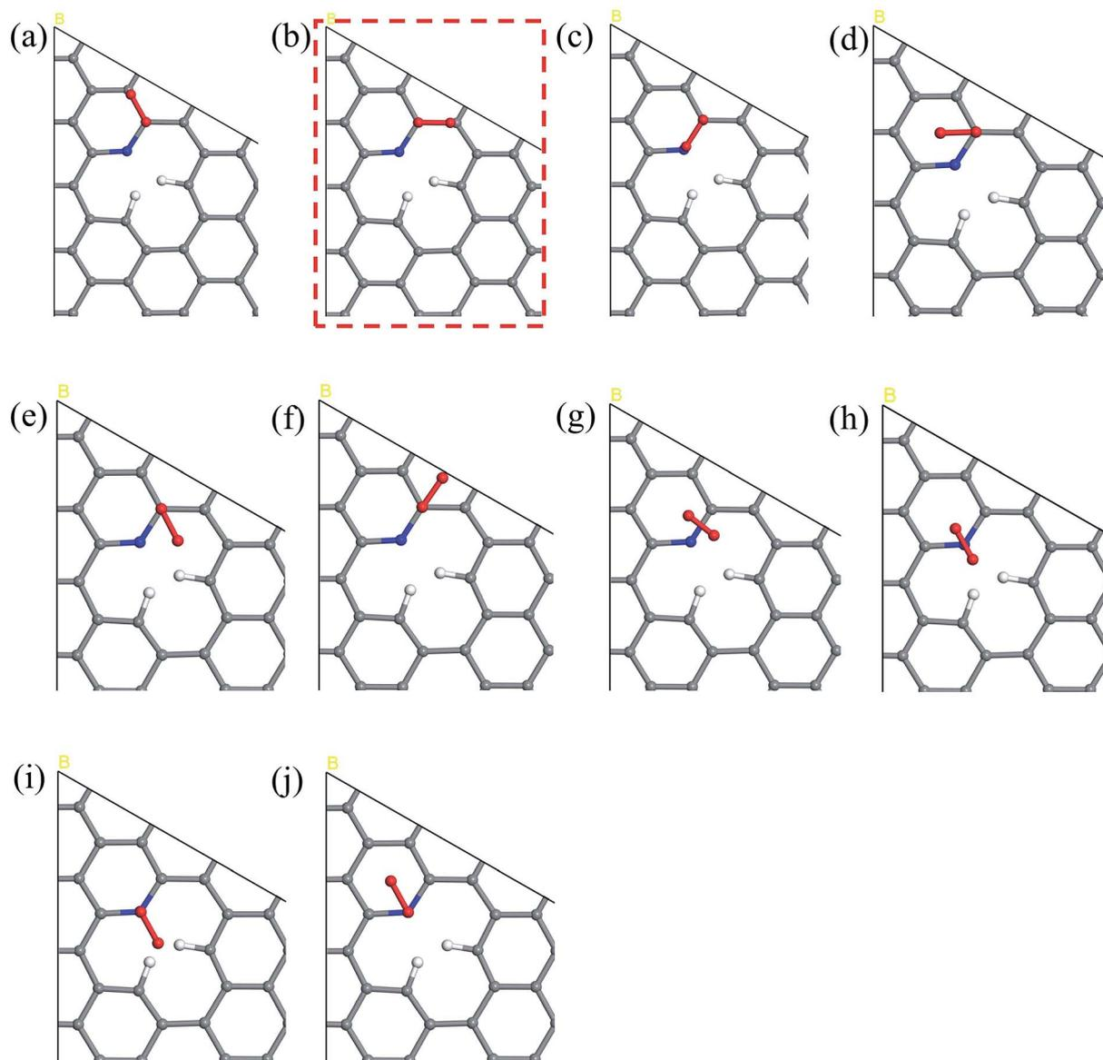
Fig. 2 The potential sites where  $O_2$  can be located on the N6 substrate for the first step of the ORR. N6\_S1\_(a) CBC1 (b) CBC2 (c) CBN (d) CH1 (e) CH<sub>2</sub> (f) CH<sub>3</sub> (g) HBH (h) HNH (i) NH1 and (j) NH<sub>2</sub>. The model marked by red dashed line has the lowest energy upon geometry optimization, indicating the most likely adsorption configuration and is used in the free energy diagram.
