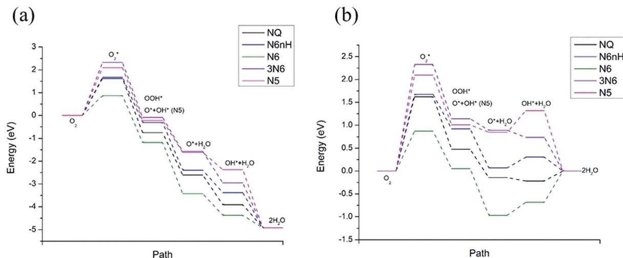
Fig. 4 Free energy diagram at (a)  $U_0 = 0$  V (vs. NHE) and (b) at  $U_{eq} = 1.23$  V (vs. NHE). Reaction pathway is  $O_2, O_2^*, OOH^*, O^* + H_2O, OH^* + H_2O, 2H_2O$ .
