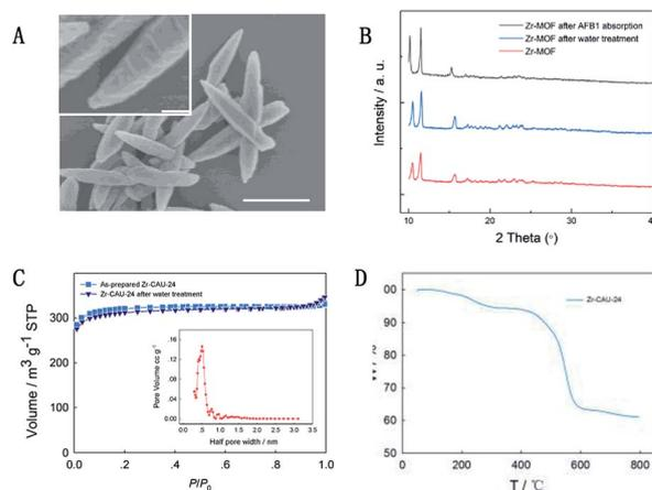
Fig. 2 Scanning electron microscopy images of prepared Zr-CAU-24 crystals with different magnification times. Scale bar: 1  $\mu\text{m}$  (A, inset). PXRD of Zr-CAU-24 crystals before and after water treatment and AFB1 absorption, (B) and  $\text{N}_2$  adsorption/desorption isotherms (C) of Zr-CAU-24 crystals before and after 24 h water treatment. TGA result of as-prepared Zr-CAU-24 crystals (D).
