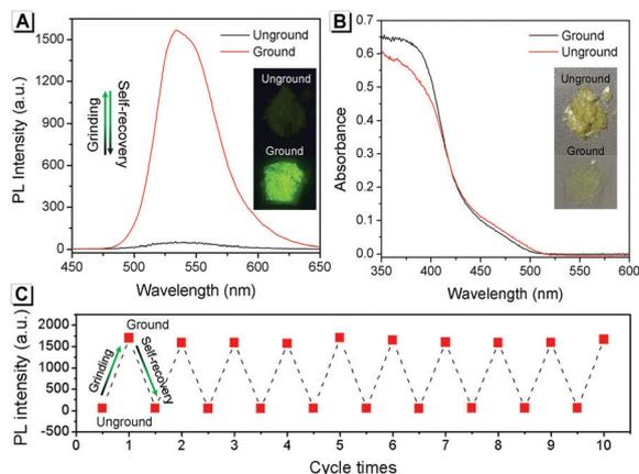
**Fig. 2** (A) Fluorescence and (B) UV-vis diffuse reflectance spectra of **SBA** before and after grinding. (C) Fatigue resistance of the fluorescence intensity of **SBA** during 10 grinding/self-recovery cycles. All spectra were recorded at 0 °C.
