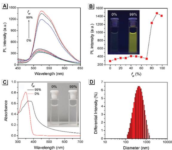
**Fig. 1** (A) Fluorescence spectra of **SBA** in water/ethanol mixtures with different  $f_w$ . (B) Fluorescence intensity of **SBA** at 525 nm as a function of  $f_w$ . (C) Absorption spectra of **SBA** in water/ethanol mixtures with  $f_w$  of 0% and 99%. (D) DLS result of **SBA** in water/ethanol mixtures with an  $f_w$  of 99%. Inset: A photo of **SBA** in water/ethanol mixtures with  $f_w$  of 0% and 99%; (B) under UV light irradiation and (C) under daylight.
