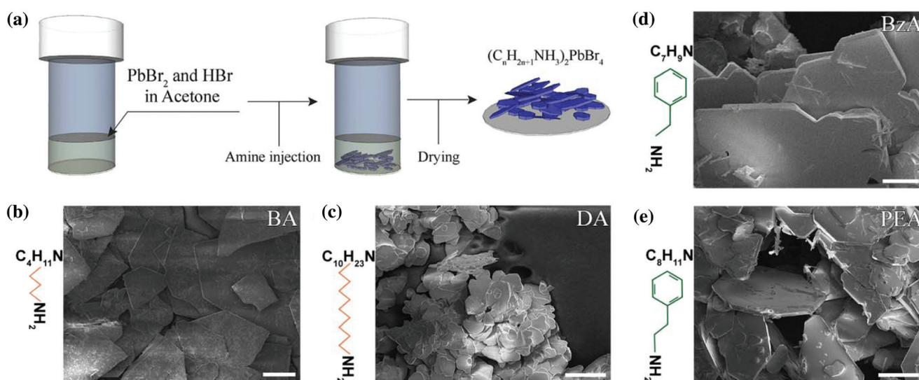
**Fig. 1** (a) Schematic diagram of the facile fabrication process of the layered perovskite by injecting a primary amine to a mixture of PbBr<sub>2</sub> in HBr and acetone. (b–e) SEM images of the produced platelets when using short and long aliphatic molecules, such as butylammonium (BA) (b) and decylammonium (DA) (c), and aromatic ones as benzylammonium (BzA) (d) and phenethylammonium (PEA) (e). Scale bars: 100 μm.
