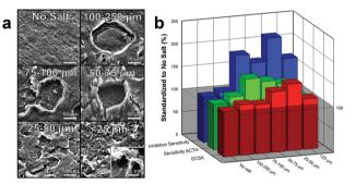
Effects of various size salt crystals for macroscale pore formation. (a) SEM depicting various size salt pores made with decreasing size salt crystals. Bottom right: Magnification of <25  $\mu m$  pore. (b) Graph demonstrated the effects of different size salt crystals to ECSA (red), sensitivity to 5 mM ACTH (green), and inhibition sensitivity due to 1 μM paraoxon (blue). Note: graph has been standardized to no salt pores for comparison.
