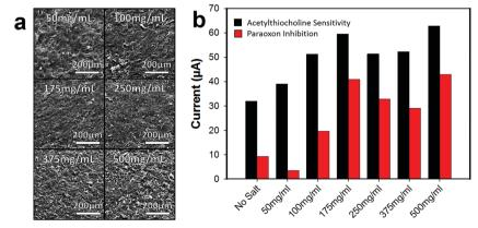
Fig. 5 Effects of various salt concretions in graphene ink. (a) Representative SEM depicting concentrations of salt forming sparse to dense pore arrays in the graphene. (b) Graph demonstrated the effects of different concentrations of salt for sensitivity to 5 mM ACHE (Black), and inhibition sensitivity due to 1 mM paraoxon (Red).
