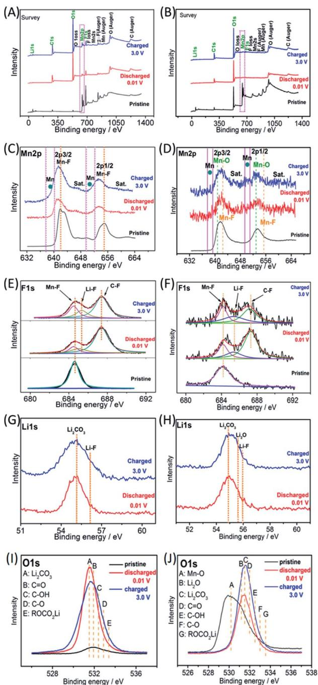
Fig. 8 *Ex situ* XPS spectra of  $\text{MnF}_2$  8# and  $\text{MnF}_2$  8#-E electrodes in the pristine, charged 3.0 and discharged 0.01 V states during the first discharging/charging cycle at  $0.05 \text{ A g}^{-1}$  for Li-ion storage: survey (A and B), Mn 2p (C and D), F 1s (E and F), Li 1s (G and H) and O 1s (I and J), respectively.
