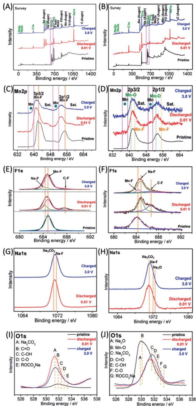
Fig. 9 *Ex situ* XPS spectra of MnF<sub>2</sub> 8# and MnF<sub>2</sub> 8#-E electrodes in the pristine, charged 3.0 V and discharged 0.01 V states during the first discharging/charging cycle at 0.02 A g<sup>-1</sup> for Na-ion storage: survey (A and B), Mn 2p (C and D), F 1s (E and F), Na 1s (G and H) and O 1s (I and J), respectively.
