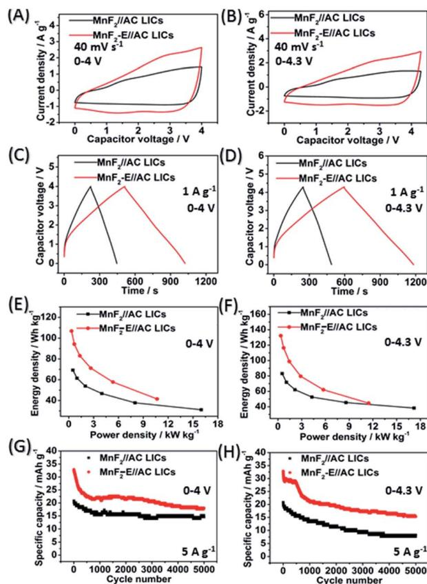
Fig. 5 CV plots at  $40 \text{ mV s}^{-1}$  (A and B), GCD curves at  $1 \text{ A g}^{-1}$  (C and D), Ragone plots (E and F) and cycling behavior for 5000 cycles at  $5 \text{ A g}^{-1}$  (G and H) of the  $\text{MnF}_2\text{//AC}$  and  $\text{MnF}_2\text{-E//AC}$  LICs under the voltages of 0–4 V and 0–4.3 V, respectively.
