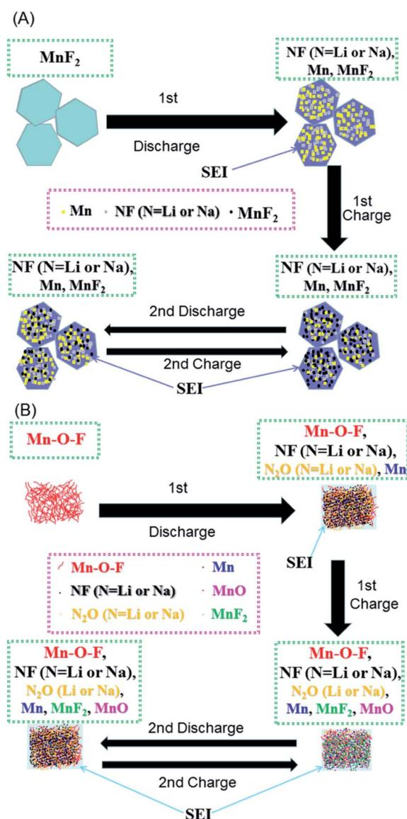
Scheme 1 Schematics of the possible reaction mechanisms for the MnF<sub>2</sub> (A) and MnF<sub>2</sub>-E (B) electrodes during the first two cycles of discharging/charging processes.
