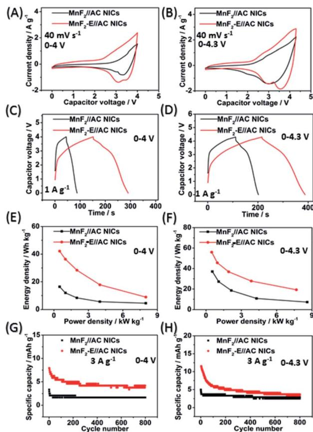
Fig. 7 CV plots at  $40 \text{ mV s}^{-1}$  (A and B), GCD curves at  $1 \text{ A g}^{-1}$  (C and D), Ragone plots (E and F), and cycling behavior for 800 cycles at  $3 \text{ A g}^{-1}$  (G and H) of  $\text{MnF}_2$  8#//AC and  $\text{MnF}_2$  8#-E//AC NICs under the voltages of 0–4 V and 0–4.3 V, respectively.
