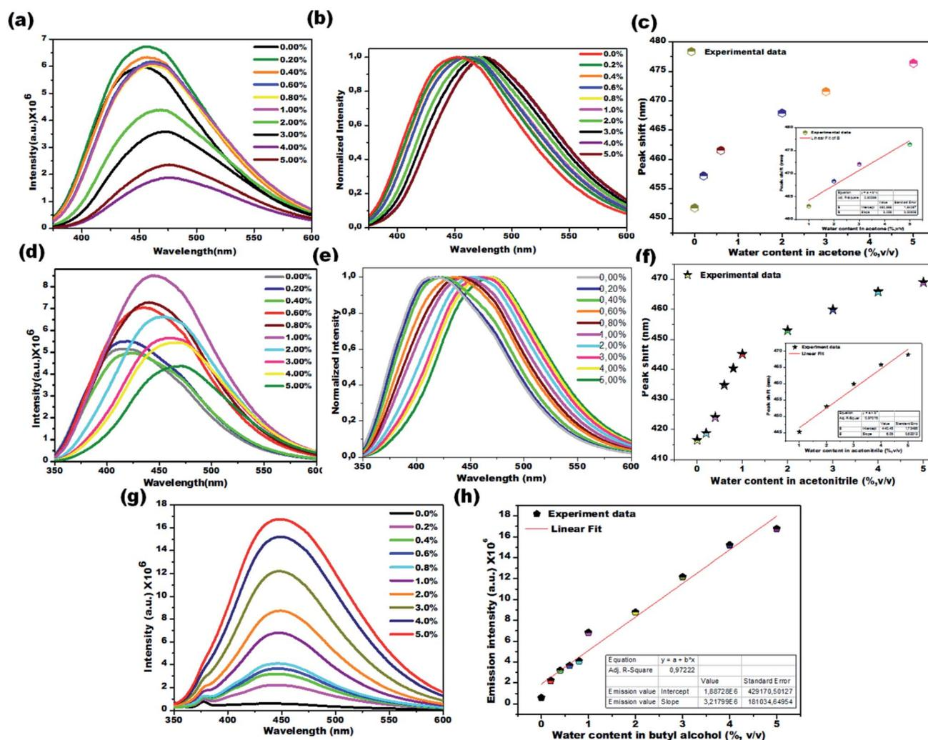
Fig. 6 Colorimetric detection of water in acetone (a–c) acetonitrile (d–f), and butyl alcohol (g and h). PL emission spectra of CD1 on varying the water content from 0.2% to 5.0% v/v (emission spectra–a, d and g: normalized emission spectra: b and e) and their calibration curve (percentage of water content vs. peak shift, c, f and h).
