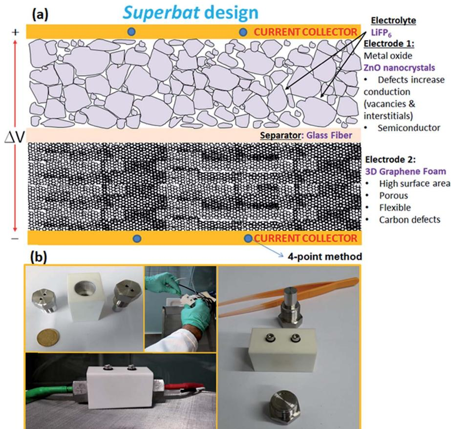
Fig. 1 (a) The *superbat* design consisting of four basic components. Advanced functional electrodes: 3D graphene foam and ZnO nanocrystals, separator: glass fiber, and electrolyte: 1 M LiPF<sub>6</sub> in EC/MC = 50/50. (b) The homemade capacitor mounting system.
