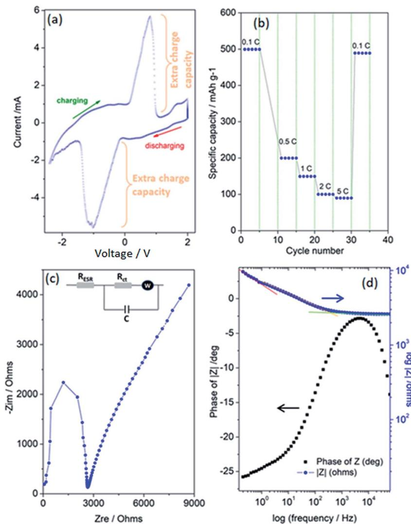
Fig. 5 Electrochemical performance results of the *superbat* designed with ZnO nanocrystal and graphene foam electrodes, LiPF<sub>6</sub> electrolyte, and a glass fiber separator. (a) Cyclic voltammety (CV), (b) rate performance obtained from the galvanostatic cycle with potential limitation (GCPL) technique. (c) Nyquist plot and (d) Bode plot obtained from electrochemical impedance spectroscopy (EIS).
