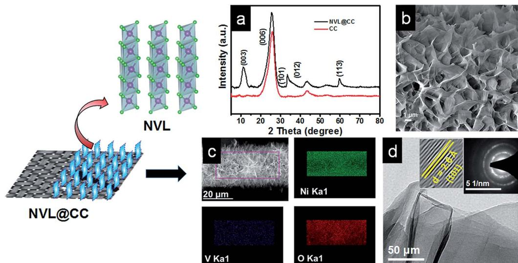
Fig. 1 (a) XRD spectra of CC and NVL@CC; (b) FESEM image of NVL@CC; (c) elemental mapping of Ni, V, and O corresponding to the area selected; (d) TEM image of NVL@CC; inset: HRTEM image and SAED pattern for NVL@CC.
