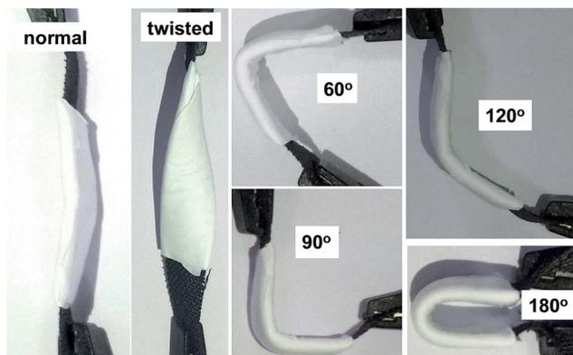
Fig. 6 Digital photographs of the NVL@CC//AC HSC at a various bending angles and in the twisted state.
