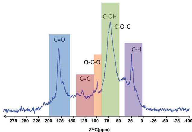
Fig. 5  $^{13}\text{C}$  MAS NMR spectrum of CDs.
