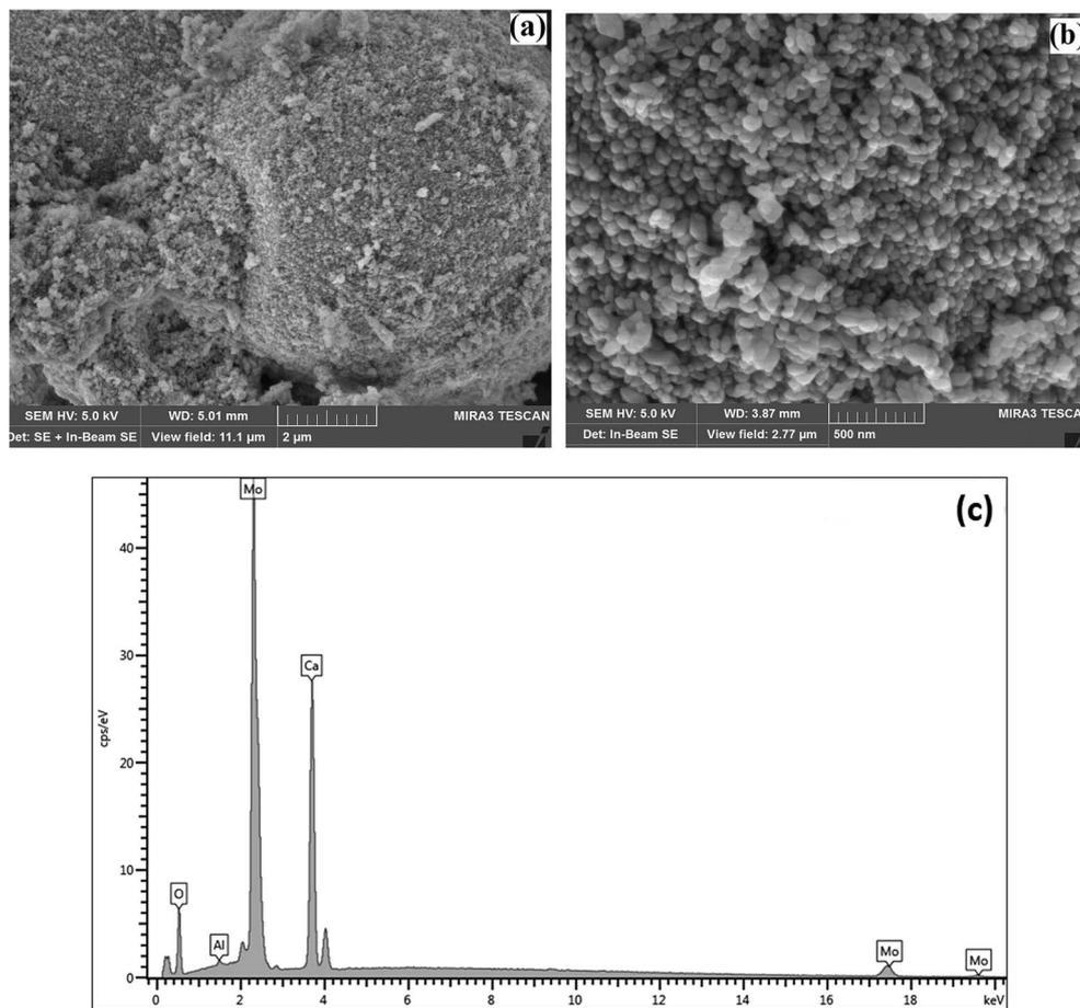
Fig. 6 SEM secondary electron images of the  $\text{CaMoO}_4$  synthesised at 300 °C showing: (a) a low magnification view of dense agglomerates of small spherical particles; (b) details of (a) showing the rounded particles to be 120–100 nm in diameter with fine scale pores between them; (c) EDS analysis showing the elemental composition of Ca, Mo, and O.
