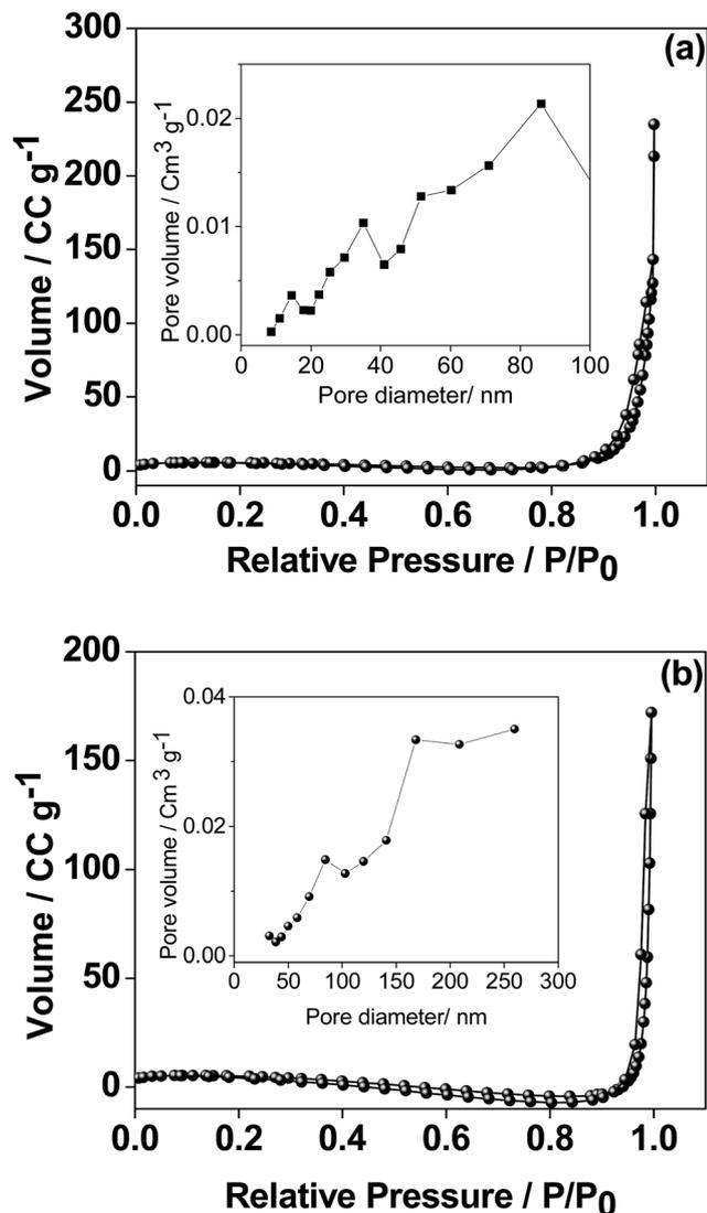
Fig. 10 Nitrogen adsorption and desorption isotherms and inset BJH adsorption pore size distribution of  $\text{CaMoO}_4$  synthesized at (a) 300 and (b) 500 °C. The isotherms for the two are quite similar while the pore size distribution is quite different – note different pore diameter scaling in the insets.
