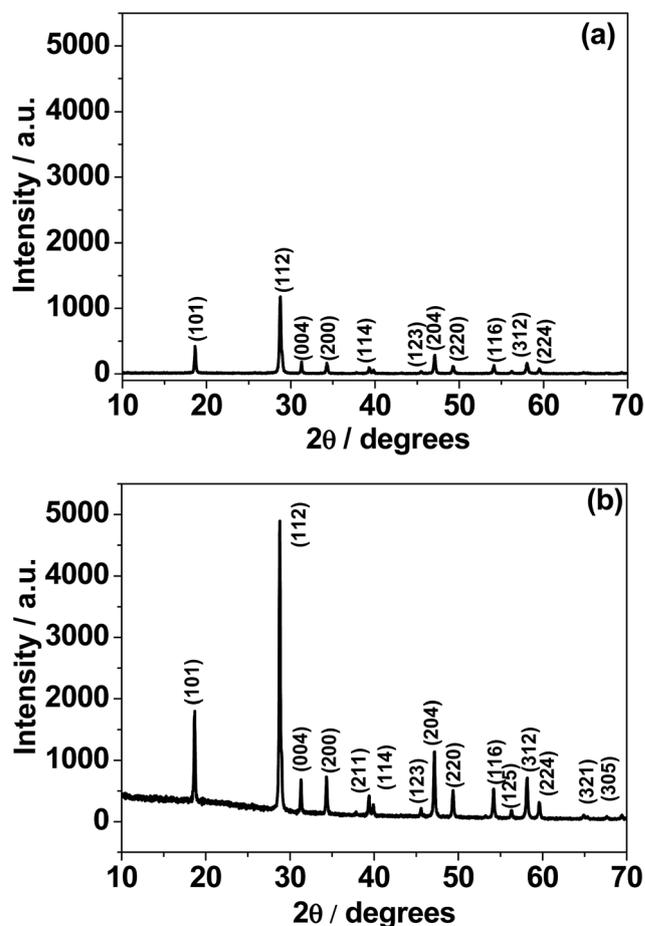
Fig. 1 X-ray diffraction (XRD) patterns of  $\text{CaMoO}_4$  synthesized at: (a) 300 and (b) 500 °C. The lower temperature material displayed a much weaker pattern, suggesting that it was not as crystalline as the higher temperature counterpart.
