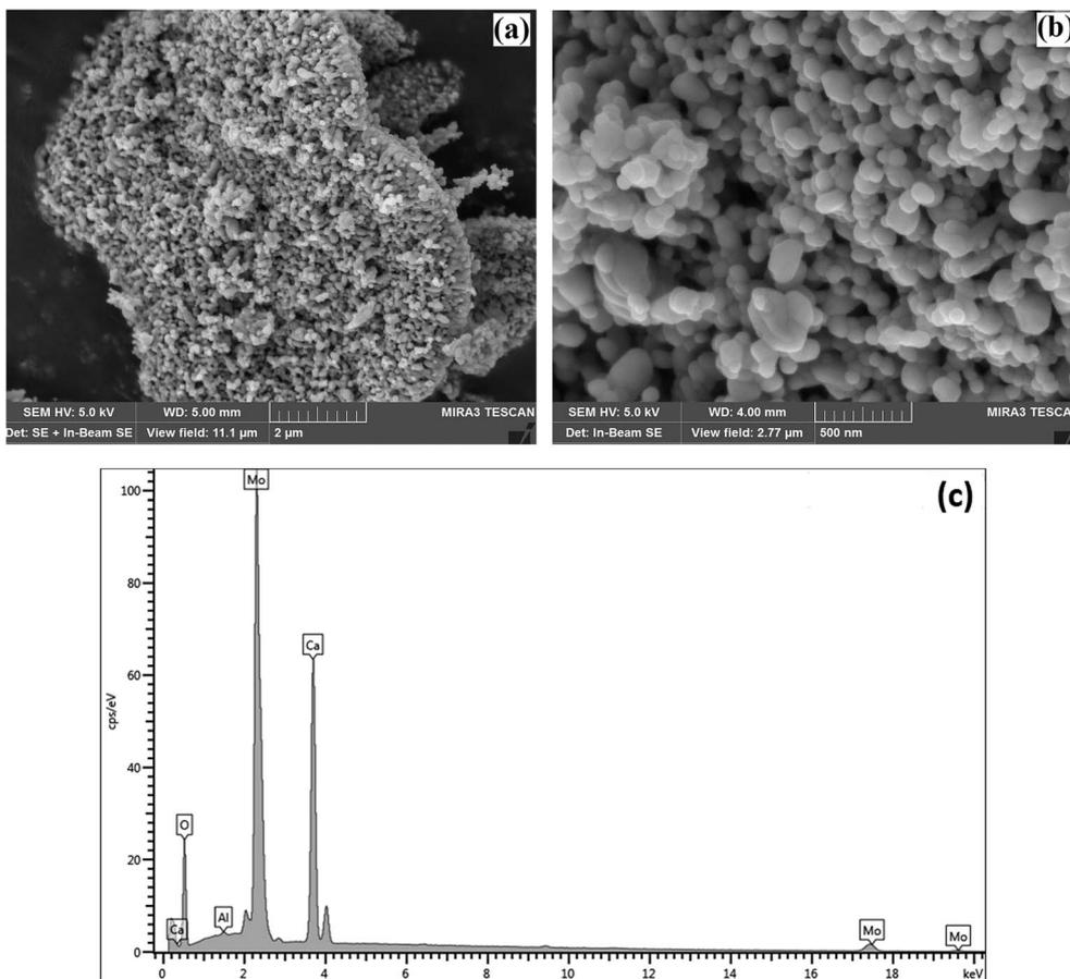
Fig. 7 (a) SEM secondary electron images of the  $\text{CaMoO}_4$  synthesised at  $500^\circ\text{C}$  showing: (a) a low magnification view of dense agglomerates of irregular-shaped particles; (b) details of (a) showing the rounded and elongated particles to be 50–250 nm in diameter with coarser scale pores between them; (c) EDS analysis showing the elemental composition of Ca, Mo, and O.
