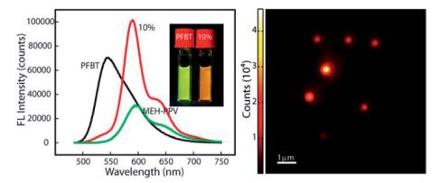
Fig. 5 (Right) PL spectra of PFBT, MEH-PPV and doped nanoparticles. Redshifted emission through efficient energy transfer in nanoparticles using PFBT as a host (energy donor) doped with a limited amount of MEHPPV (energy acceptor). (Left) AFM image of doped-nanoparticles. Adapted with permission from ref. 79. Copyright 2013 American Chemical Society.
