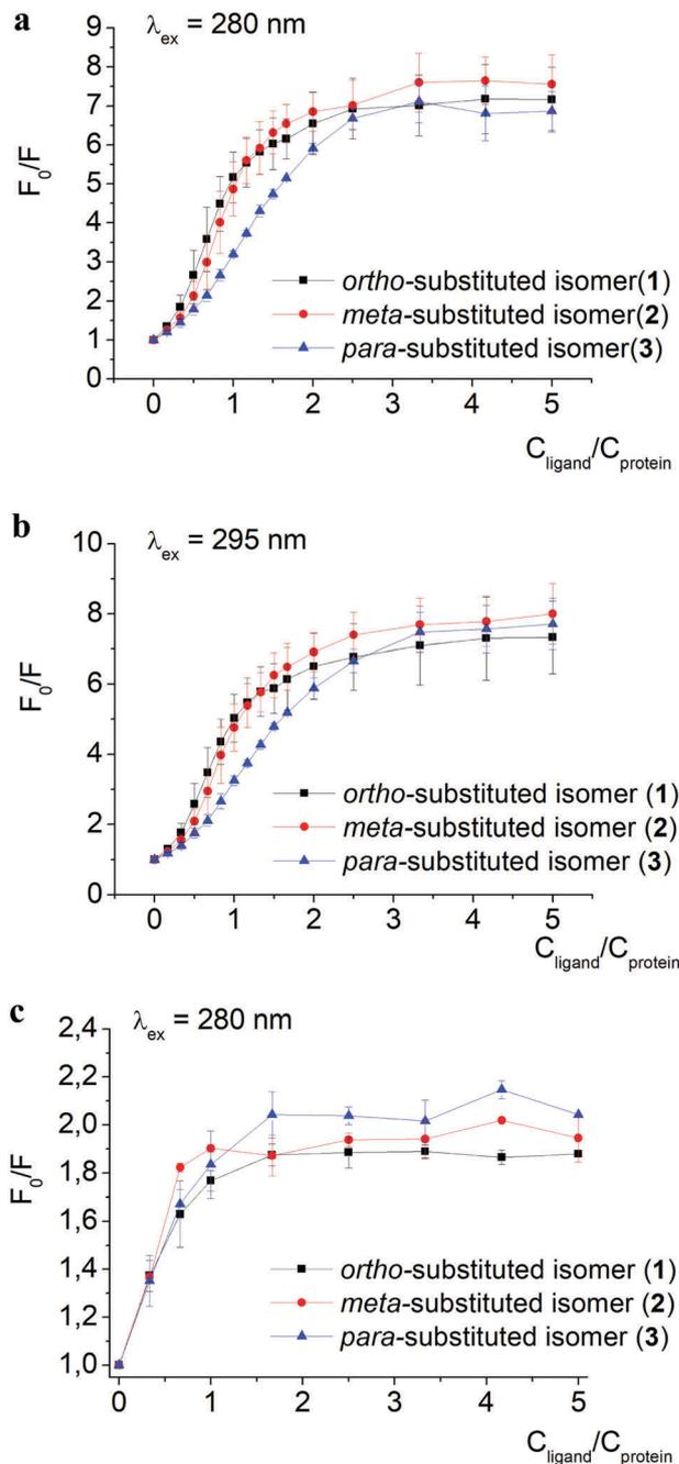
Fig. 2 Stern–Volmer plots of fluorescence intensity quenching of BSA emission excited at 280 (a) and 295 (b) nm, as well as of HSA emission excited at 280 nm (c), by clathrochelates **1–3**;  $F_0$  and  $F$  are protein fluorescence intensities in the absence and in the presence of these complexes. Spectra were recorded in 0.05 M Tris HCl, pH 7.9.
