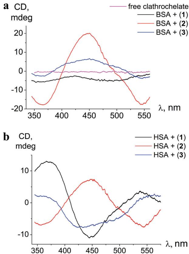
Fig. 3 ICD spectra of clathrochelates 1–3 in the presence of BSA (a) and HSA (b);  $C_{\text{albumin}} = 8 \times 10^{-5} \text{ mol l}^{-1}$ ,  $C_{\text{clt}} = 4 \times 10^{-5} \text{ mol l}^{-1}$ . Spectra are recorded in 0.05 M Tris HCl pH 7.9.
