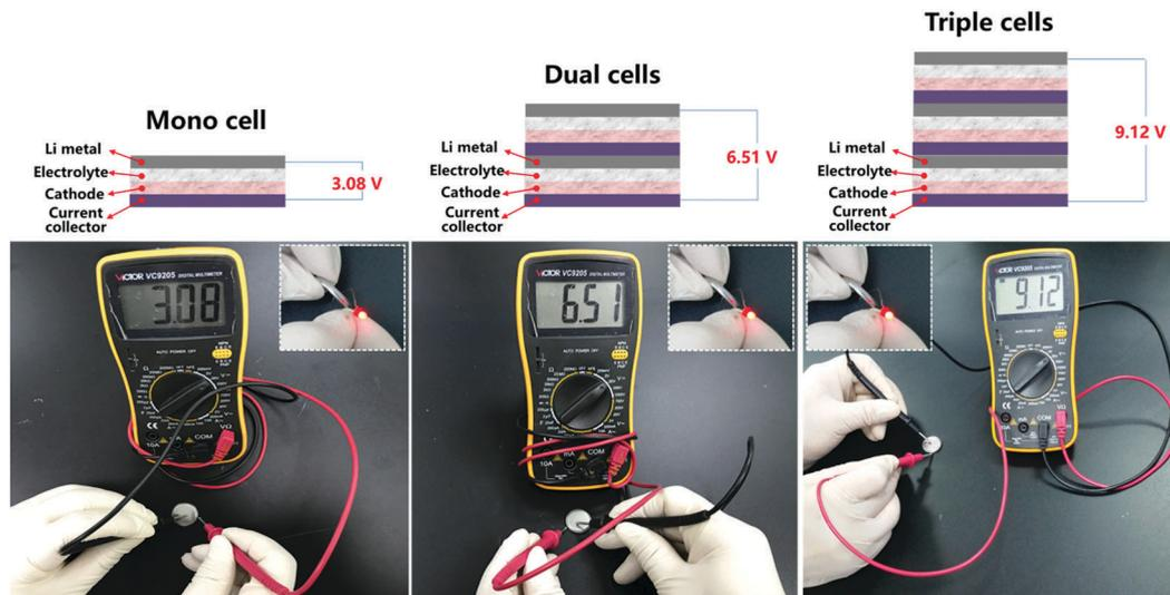
Fig. 5 A cathode-supported SSLIB showing a VOC of 3.08 V, a battery pack made by two cathode-supported SSLIBs showing a VOC of 6.51 V, and a battery pack made by three cathode-supported SSLIBs showing a VOC of 9.12 V. All mono/dual/triple cells can power LED light.
