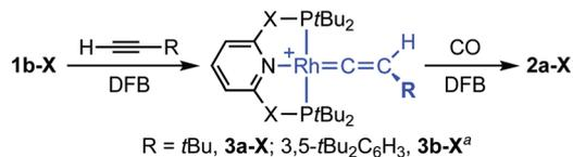
**Scheme 3** Preparation of vinylidene complexes **3** (X = O, CH<sub>2</sub>). [Bar<sup>F</sup><sub>4</sub>]<sup>−</sup> counter anions omitted for clarity; <sup>a</sup> **3b-O** formed as mixture with the corresponding  $\pi$ -complex **2e-O**.
