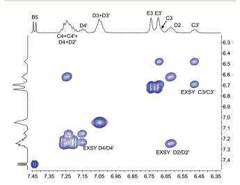
Fig. 7 Part of the NOESY spectrum (500 MHz, acetone- $d_6$ ) of [Cu(xantphosMes<sub>2</sub>)(6-Mebpy)][PF<sub>6</sub>] showing exchange (EXSY) peaks between pairs of protons C3 and C3′, D2 and D2′, and D4 and D4′. See also Fig. S20.†
