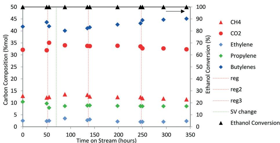
Fig. 8 Ethanol conversion (mol%) and product selectivity (mol C%) over  $Zn_1Zr_{2.5}O_z$  (50 wt% ethanol in water feed; 450 °C, 1.38 MPa,  $GHSV = 320$  to  $660$  h<sup>-1</sup>). Vertical red dotted lines represent regeneration steps and green dotted line marks a change in contact time.
