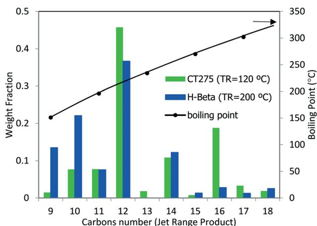
**Fig. 12** Carbon number distribution as determined by GC-MS for the reaction product *via* sequential oligomerization shown in Fig. 11 followed by hydrotreatment. Right axis (black line) indicated the average boiling point. Hydrotreated products comprised primarily paraffins with less than 0.3 area% of other compounds. No aromatic compounds were detected.
