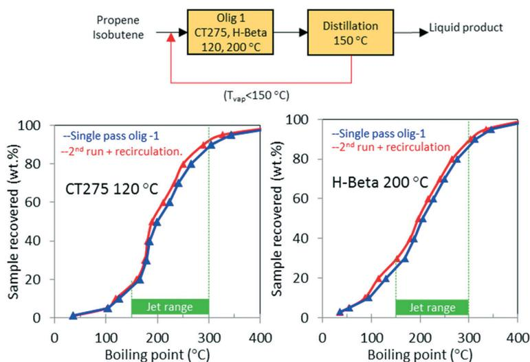
**Fig. 10** Simulated distillation results for the reaction product of model isobutene/propene (4/1 molar) feed mixture over H-beta (left side) and CT275 (right side) after single-pass conversion (blue line) and for a second run (red line) incorporating the light olefins of the first run (b.p. < 150 °C).
