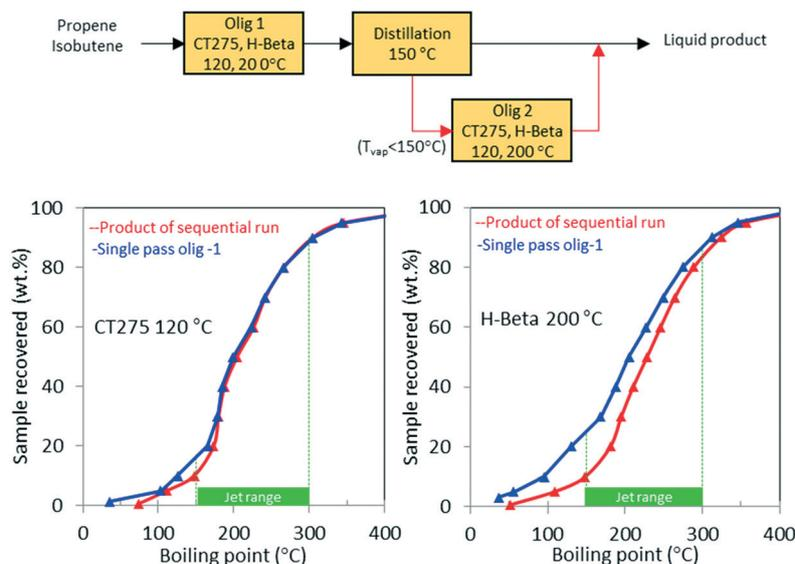
**Fig. 11** Simulated distillation results for the reaction product of model isobutene/propene (4/1 molar) feed mixture over H-beta (left figure) and CT275 (right figure) after single-pass conversion (blue line) and after a second oligomerization (red line) of the light olefins obtained in the first run (b.p. < 150 °C).
