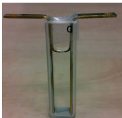
Fig. 8 (a) The parallel-rod arrangement of Radacsi, 59 along with the schematic representation of the scheme and (b) the parallel-plate arrangement with the equivalent schematic. Reprinted with permission from ref. 59.
