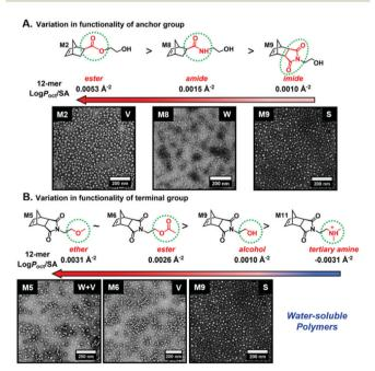
Fig. 2 Oligomer  $log P_{oct}$ /SA values as a function of (A) anchor and (B) terminal group variations for NB-based monomers suitable for use as core-forming blocks during aqueous ROMPISA, and representative nanoobject TEM images for corresponding diblock copolymers of approximately the same length. Adapted with permission from ref. 59. Copyright 2019 American Chemical Society
