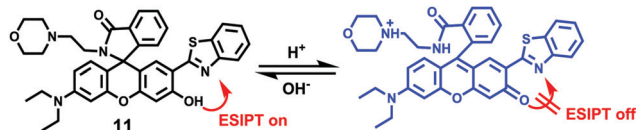
Scheme 8 Fluorescent probe 11 for pH.
