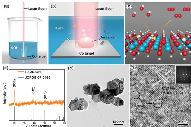
**Fig. 1** Synthesis and characterization of L-CoOOH. (a) Schematic illustration of the synthesis of L-CoOOH via LAL and (b) the corresponding magnification of the laser irradiation region. (c) Schematic representation of L-CoOOH with abundant oxygen vacancies for the OER. Color code: white for H, red for O, cyan for Co, and transparent color for vacancy. (d) XRD pattern of L-CoOOH. (e and f) Low-magnification TEM and HRTEM images of L-CoOOH. The inset in (f) shows the SAED pattern of L-CoOOH.
