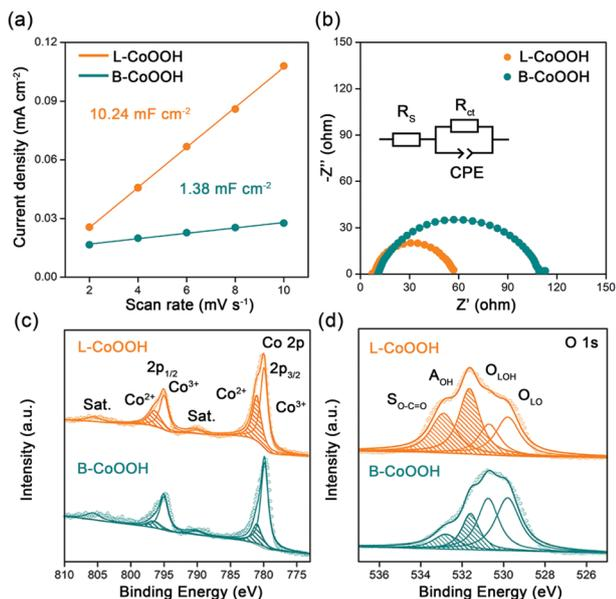
Fig. 3 Origin of the excellent OER activity of L-CoOOH. (a) The relationship between the current density and the scan rate. (b) The EIS of L-CoOOH and B-CoOOH recorded at a potential of 1.56 V<sub>RHE</sub>. (c) Co 2p and (d) O 1s XPS spectra of L-CoOOH and B-CoOOH.
