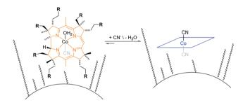
Fig. 1 Schematic overview of cyanide binding with immobilized corrinoids in the detection zone of the CyanoKit.  $R = COOC_nH_{2n+1}$  where n = [1,4].
