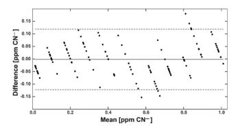
Fig. 6 Bland-Altman plot comparing the ground truth of the cyanidespiked H<sub>2</sub>O with the smartphone measurements. The continuous line depicts the mean error and the dashed lines enclose the 95% confidence interval.
