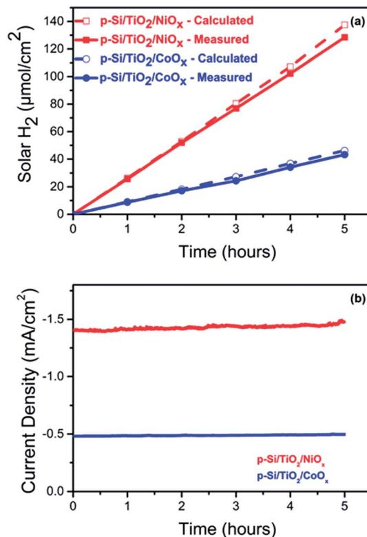
Fig. 4 Comparison of (a) the calculated and measured solar hydrogen production per geometric surface area of the photoelectrode and (b) of the current density of  $\text{NiO}_x$  (red) and  $\text{CoO}_x$  (blue) functionalized p-Si photo-electrodes over 5 hours of continuous operation. The data displayed in (a) and (b) were obtained simultaneously at  $0.0 V_{\text{RHE}}$  and 1 sun illumination.
