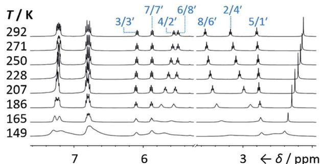
**Fig. 2** Partial <sup>1</sup>H NMR spectra (500 MHz, CS<sub>2</sub>-CD<sub>2</sub>Cl<sub>2</sub>) of **1b/1b'**. As the temperature is decreased, the equilibrium shifts towards the lower-energy isomer **1b**. At temperatures below 186 K, the broadening of peaks indicates the reversible Cope rearrangement is entering the slow-exchange regime. Selected resonances are labelled according to the numbering in Scheme 1.
