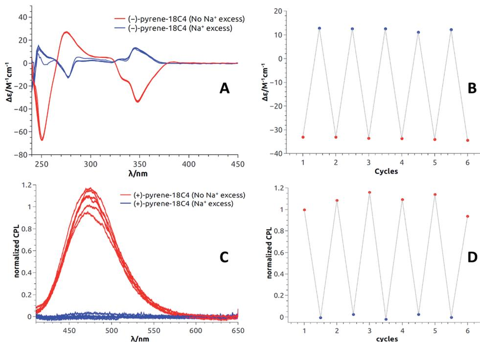
Fig. 8 **Pyrene-18C4** (CH<sub>2</sub>Cl<sub>2</sub>): Reversible ECD ((A) first eluted (–)-enantiomer) and intensities at 348 nm (B). Reversible CPL ((C) second eluted (+)-enantiomer) and normalized intensities at 480 nm (D).
