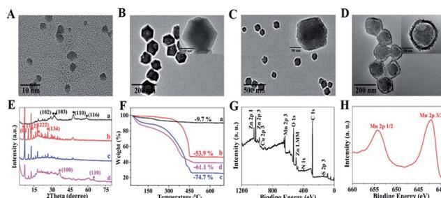
**Fig. 1** TEM images of (A) CuS, (B) CuZ, (C) CuZP, and (D) CuZPMn (inset: the enlarged TEM images). (E) XRD patterns and (F) TGA of (a) CuS, (b) CuZ, (c) CuZP, and (d) CuZPMn. (G) XPS spectrum of CuZPMn and (H) high-resolution Mn 2p XPS spectrum (Cu, Z, P, and Mn in CuZPMn represent CuS, ZIF-8, polydopamine, and MnO<sub>2</sub>, respectively. The abbreviations are also listed in ESI Table S1†).
