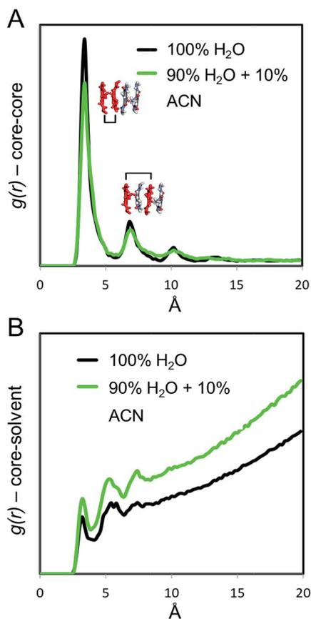
Fig. 6 Radial distribution functions  $g(r)$  of the (A) C<sub>12</sub>BTA-cores, and of (B) C<sub>12</sub>BTA-cores–water. Both  $g(r)$  were calculated from the MD simulations in pure water (black) and in water with 10% ACN (green).
