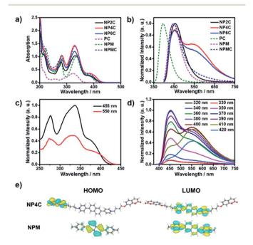
Fig. 2 (a) Absorption spectra and (b) PL emission spectra of aqueous NP2C, NP4C, NP6C, PC, NPM and NPMC solutions; (c) PL excitation spectra for dual emission of NP4C, respectively, monitored at 455 and 550 nm. (d) PL emission spectra of NP4C measured at various excitation wavelengths. (e) Calculated frontier molecular orbitals of NP4C and NPM. [NP2C] = [NP4C] = [NP6C] = [NPM] = [PC] = [NPMC] = 25  $\mu\text{M}$ .
