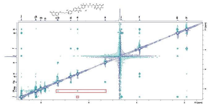
Fig. 3 2D ROESY spectrum of NP4C in  $D_2O$  with water suppression. [NP4C] = 1.0 mM, 25 °C.
