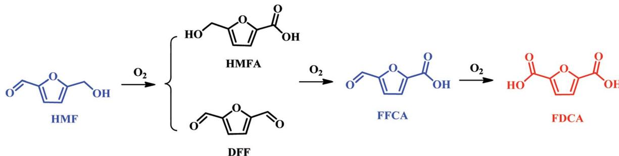
Scheme 3 Reaction pathway for aqueous HMF oxidation.
