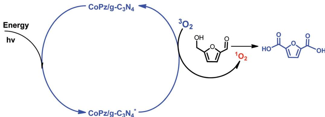
Scheme 4 Possible mechanism of the photocatalytic oxidation of HMF into FDCA with the CoPz/g-C<sub>3</sub>N<sub>4</sub> catalyst.
