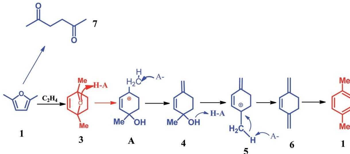
Scheme 5 Detailed reaction network of DMF and ethylene at 528 K.<sup>87</sup>
