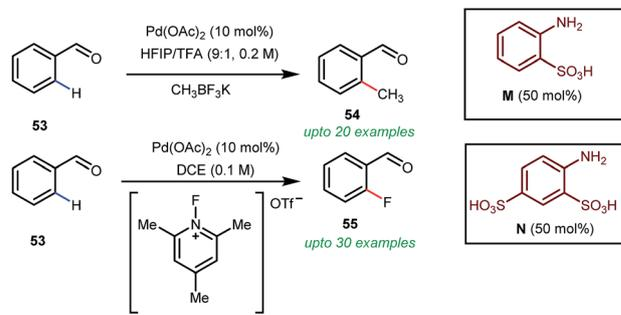
Fig. 21 Pd-catalyzed *ortho*-methylation and fluorination of benzaldehydes.
